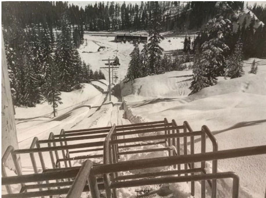
An empty Ski Boggan – showing standing area for passengers to hold onto.
